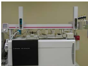
Dual rail Multipurpose sampler on LC-QQQ-MS to perform automated QuEChERS
