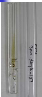
Dimpled 2mm id Liner – I have seen an improvement in reproducibility and linearity compared to helical liners
